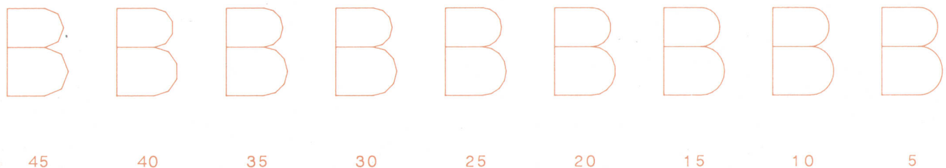
Fig. 6. Effect of chord angle on character quality. The letter B is drawn above for various selected chord angles. The smaller the chord angle the smoother the arcs and the longer it takes to write the character.
